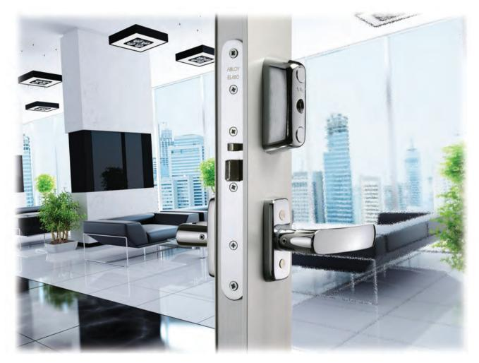
**ABLOY®** EL480 and PE480 sare especially suited for use in exit doors because inside handle (EN 179) or panic bar (EN 1125) enables egress at all times.
